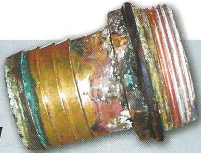
This seacock component, from John Epton's 11-year-old Bavaria 42, displays pink dezincification all round the connector
